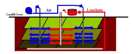
Figure 1: The Aerobic Stabilization Process at a Landfill
