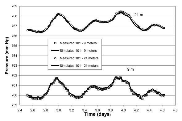
Figure 3 Measured and Simulated Pressures at Location 101 (Phase 5)
