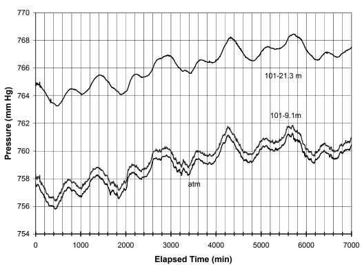
Baro-Pneumatic Data: Phase V South Cell Probe Nest 101
